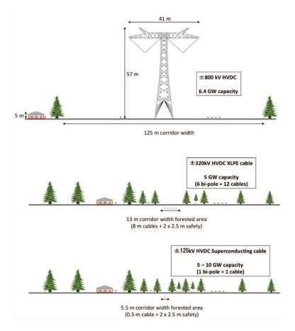
Size comparison of different technological options for electricity transmission.
