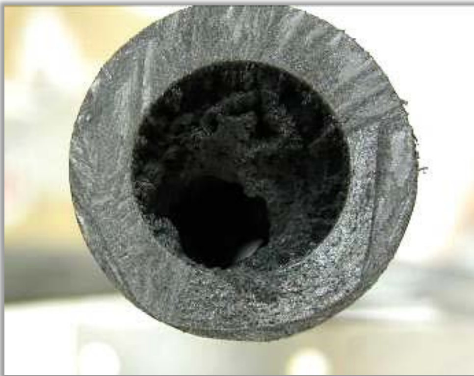
Figure 4 Carbon clogging in a tubular experimental reactor [14].
