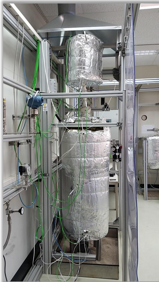
Figure 7 Photograph of the methane cracking experimental facility at KIT showing the insulated liquid metal reactor in the bottom.
