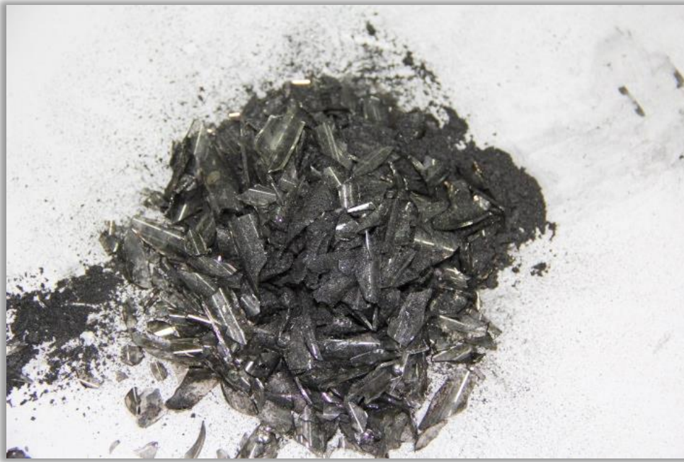
Figure 9 Carbon powder accumulated on top of the surface of the liquid metal along with quartz glass pieces that formed the packed bed.
