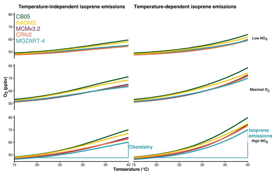
**Figure 3.** Mean ozone mixing ratios (ppbv) at each temperature after allocation to the different NO<sub>x</sub> regimes of Fig. 2a. The differences in ozone mixing ratios due to chemistry (solid line) and isoprene emissions (dotted line) are represented graphically for MOZART-4 with high-NO<sub>x</sub> conditions. Table 2 details the differences for each chemical mechanism and NO<sub>x</sub> condition.
