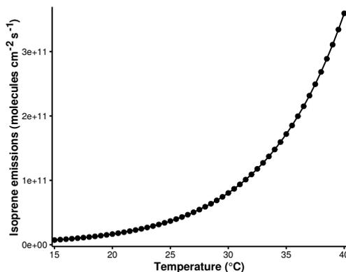
**Figure 1.** The estimated isoprene emissions (molecules isoprene cm<sup>-2</sup> s<sup>-1</sup>) using MEGAN2.1 at each temperature used in the study.
