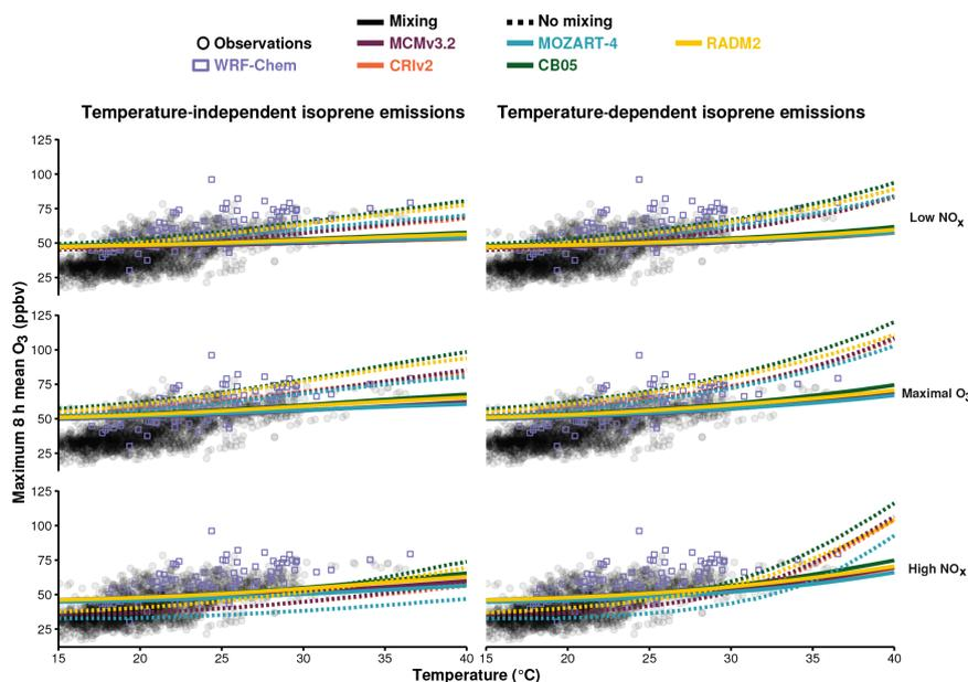
**Figure 5.** MDA8 values of ozone from the box model simulations allocated to the different NO<sub>x</sub> regimes for each chemical mechanism with mixing (solid lines) and without mixing (dashed lines). The slopes of the box model ozone–temperature correlation is compared to the summer 2007 observational data (black circles) and WRF-Chem output (purple boxes) in Table 3.
