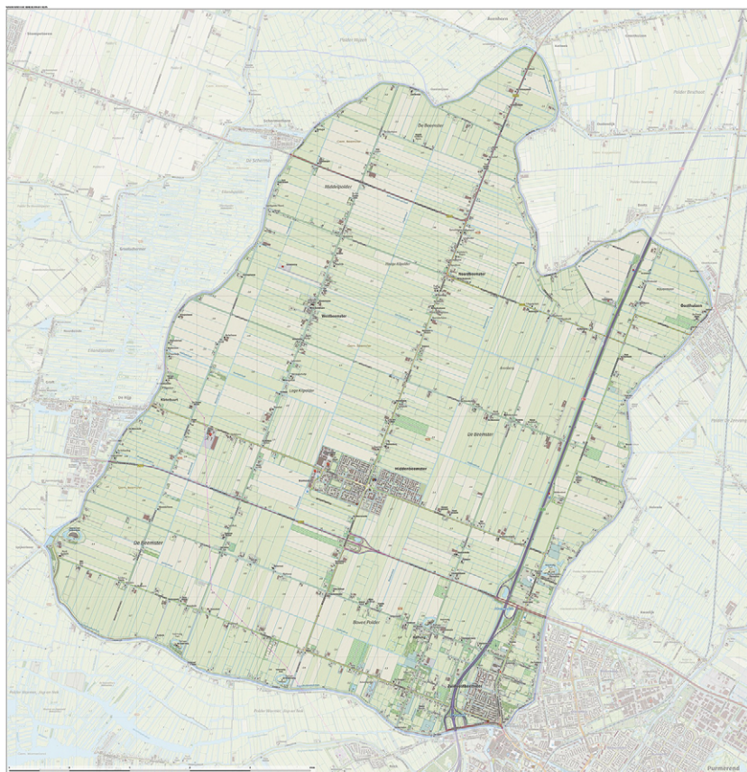
FIGURE 10.5a Topographic map of the Beemster polder in the Netherlands in 2015. One clearly sees the canal surrounding the polder, which served to drain it (and now keeps it dry), and the rectangular spatial organization of ditches that connect to the surrounding canal. At the time of drainage, the water was removed by windmills, as in Figure 10.5b; now it is removed by modern pumps. (Open access CC-BY)
