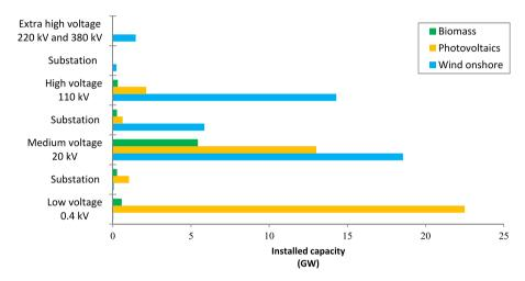
Fig. 2. Installed capacity for biomass, photovoltaics and wind energy per voltage level, calculated for the year 2015 from data in (50 Hertz et al., 2016).
