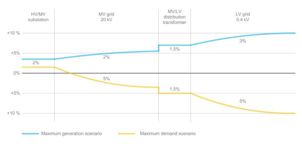
Fig. 3. Recommended allocation of voltage bandwidth, based on (Forum grid technology of the VDE, 2016).
