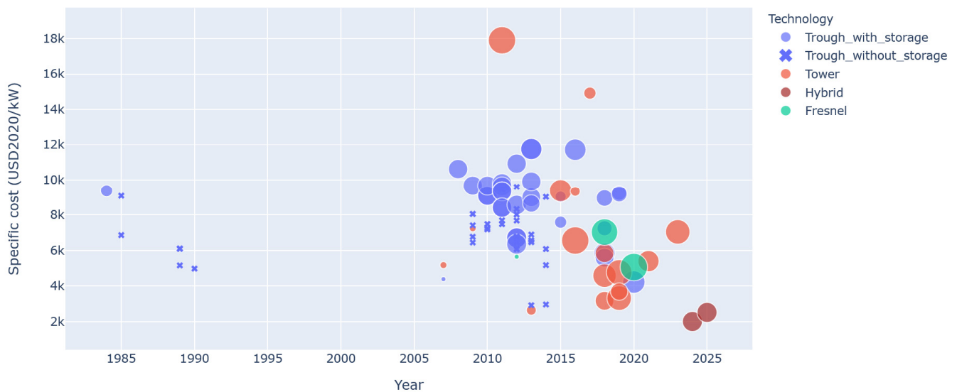
Figure 7. Specific investment costs for CSP plants since 1984 (blue: trough, red: tower, green: Fresnel, brown: hybrid plant). Circles refer to CSP plants with thermal storage with the size depending on the storage capacity. Crosses refer to CSP plants without storage.
