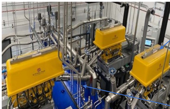
Figure 33. Stirling Cryogenics 67 K sub-cooled LN 2 cable cooling system.
